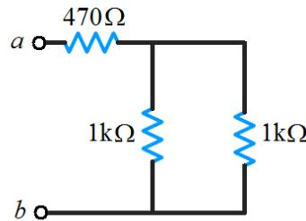
5. Build the *current divider* circuit in Figure 6 with  $R_1 = 470\Omega$  and  $R_2 = 1\text{k}\Omega$ . Use the  $+30\text{V}$  supply on the DC power source and set its supply current to  $30\text{ mA}$ . Use the multimeter to verify and monitor the value of the supply current,  $i$ . Record  $i$ . Measure and record the currents  $i_1$  and  $i_2$  in resistors  $R_1$  and  $R_2$ , respectively.
