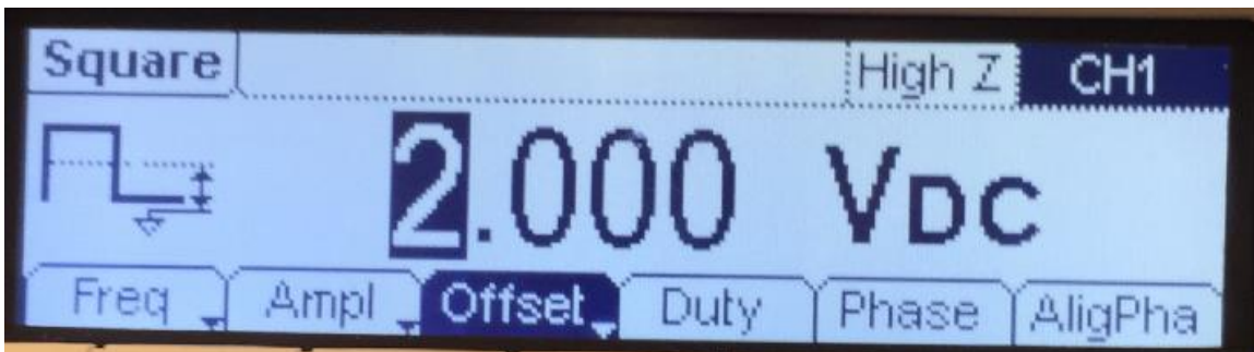
Figure 8 FG display for 2V dc bias added to a square signal.
