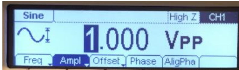
Figure 4 Default screen of the FG immediately after reset.
