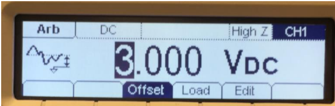
Figure 7 FG display for a DC signal.
